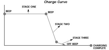
**Stage One** — Rapid Start Charge at 10 amps delivers maximum charging amperage to "wake up" any serviceable 12 volt battery and allows for quick engine starting in just 5 minutes (based on a midsize vehicle battery at 50% charge level). When battery reaches a maximum safe predetermined voltage, the charger will automatically signal a "beep" and move into Stage 2 of the charging process.
